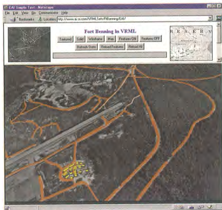
4 A tiled terrain model showing geo-referenced 3D geometry overlaid for roads (orange) and buildings (yellow).
